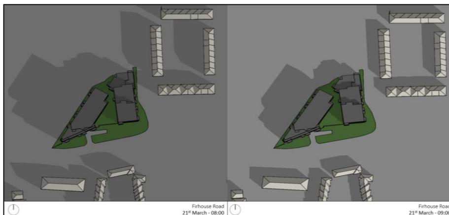
Figure 32: Overshadowing Images on March 21<sup>st</sup> at 8 a.m. and 9 a.m.
