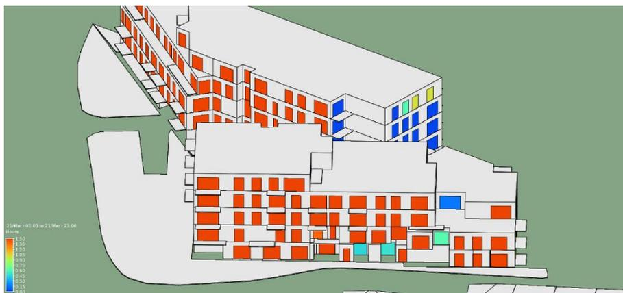
Figure 24: Sunlight Exposure March 21<sup>st</sup> (EN 17037 Min Recommendation) – East Elevation
