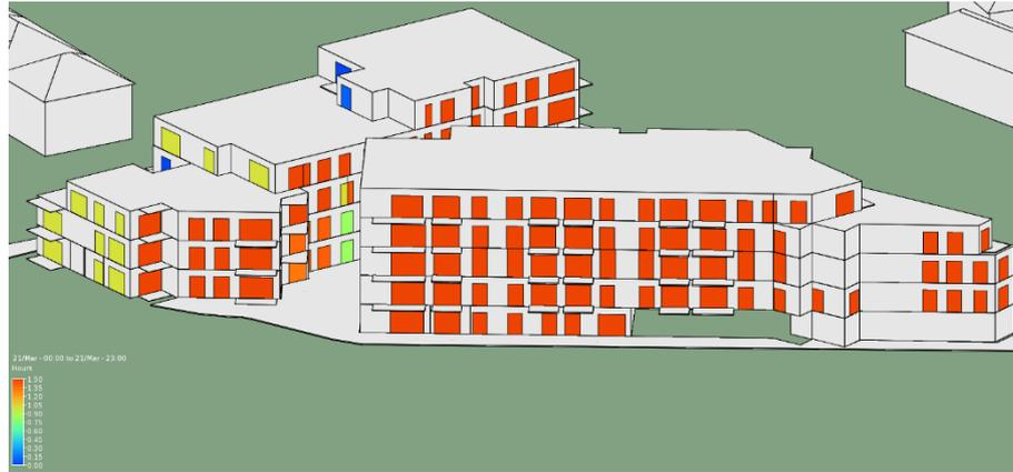
Figure 25: Sunlight Exposure March 21<sup>st</sup> (EN 17037 Min Recommendation) – North West Elevation
