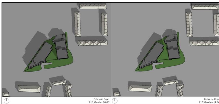
Figure 33: Overshadowing Images on March 21<sup>st</sup> at 10 a.m. and 11 a.m.
