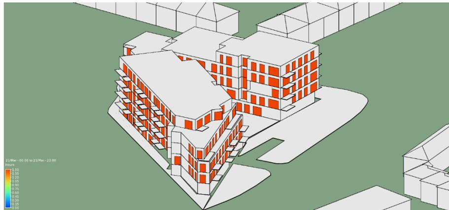
Figure 26: Sunlight Exposure March 21<sup>st</sup> (EN 17037 Min Recommendation) – South West Elevation
