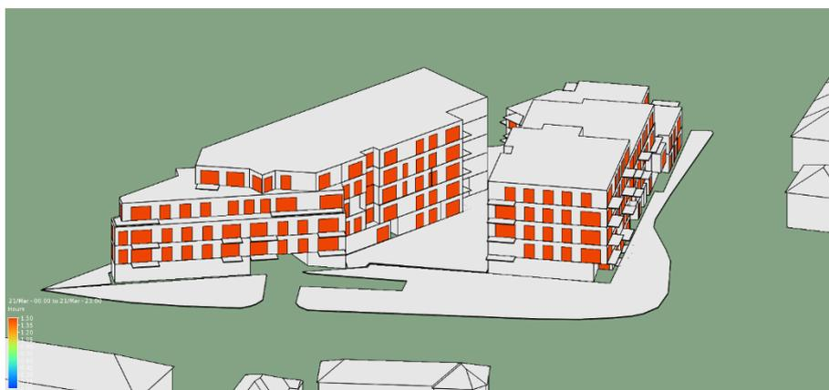
Figure 23: Sunlight Exposure March 21<sup>st</sup> (EN 17037 Min Recommendation) – South Elevation
