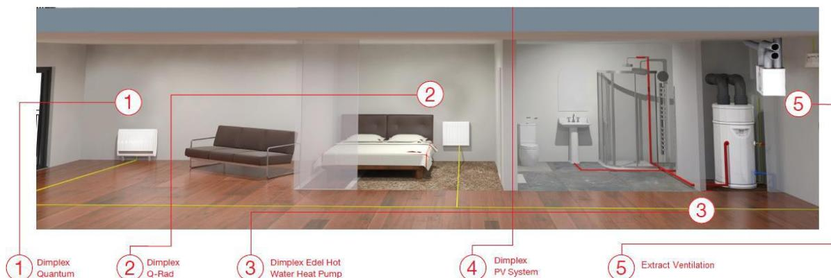
Figure 6: Typical Air-Source Heat Pump with Electric Panel Heaters Arrangement
