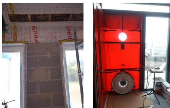
Figure 3: Air Tightness Testing Examples
